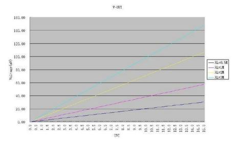
About the Xadow UV Sensor, we use a resistance which resistance value is 3M, so you need refer to this line for RL=3M. It is linear observing the relationship between voltage and UV. And the formula by calculated can be gotten: UV Index = Voltage/9.71 which has been used in code.
